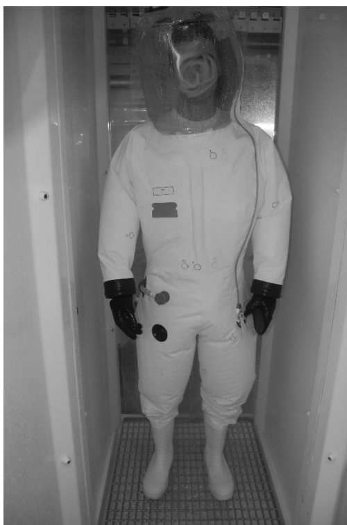
Figure 7. A Honeywell BSL-4 positive pressure suit in a decontamination shower mock up.
