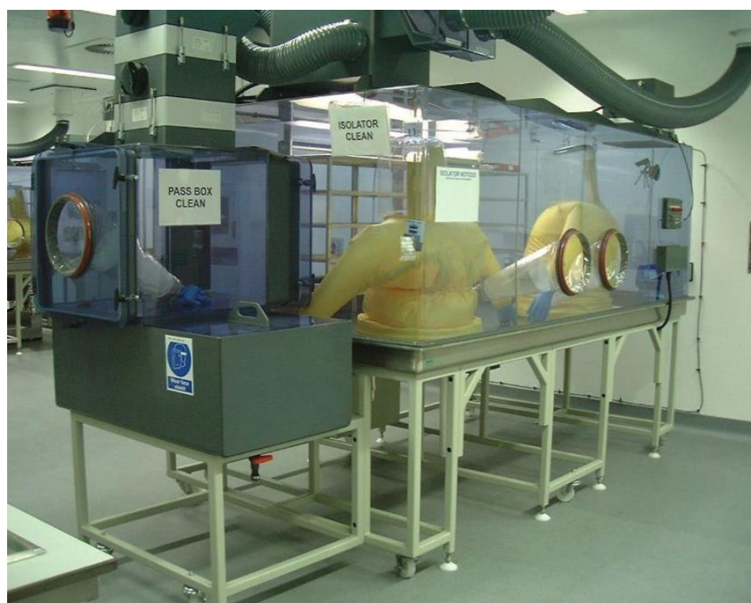
Figure 6. A solid frame isolator used in a BSL-4.
