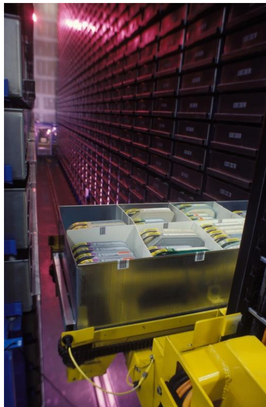
Figure 3. Example of an automated storage and retrieval system (Source: Wikimedia Commons).
